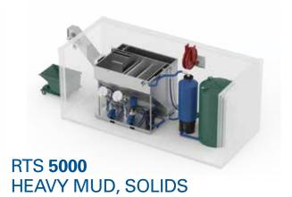
RTS 5000 is the best filtration system for heavy dirt operations. Inclined plate separators drop solids into the RTS 5000's built-in conveyor, transferring the mud to an external hopper for easy disposal. Then through a filtration filter down to 5 microns.
