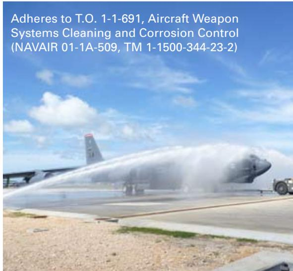
Adheres to T.O. 1-1-691, Aircraft Weapon Systems Cleaning and Corrosion Control (NAVAIR 01-1A-509, TM 1-1500-344-23-2)
